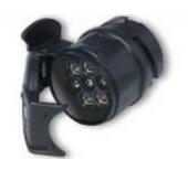
An alternative (avoiding the excess cable length issue) is a simple plug which converts a 13-pin socket to a 12N 7-pin socket. These are also useful if towing something other than a caravan, which doesn't require 12S circuits. A similar plug converts a 12N 7-pin socket to a 13-pin socket, although clearly only the road light circuits are included. Most adapters are commonly available through caravan accessory shops
